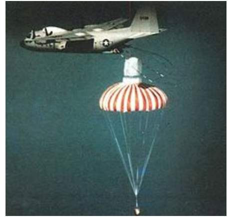
A U.S. JC-130 aircraft retrieving a reconnaissance satellite film capsule under parachute.
