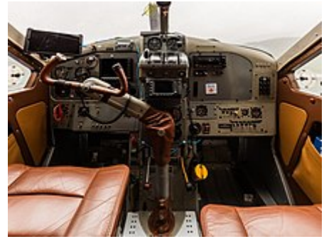
Instrument panel of a DHC-2 – note the single pilot's yoke, that can be handed over to the co-pilot, in flight.
