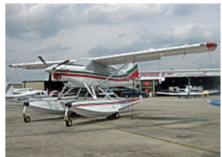
Wipaire Boss Beaver conversion with PT6 turbine engine, retaining original fin shape and fitted with floats, at Bartow Municipal Airport, Florida in 2011
