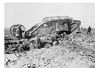
British First World War Mark I tank; the guidance wheels behind the main body were later scrapped as unnecessary. Armoured vehicles of the era required considerable infantry and artillery support. (Photo by Ernest Brooks)
